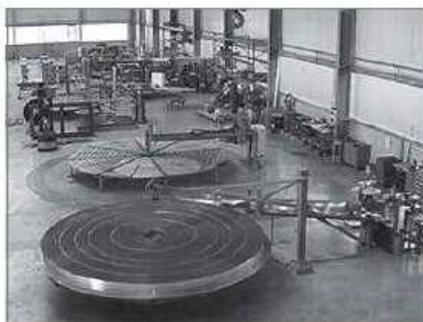
Fig. 9: A corrugated and a smooth metal foil are wound around each other.
