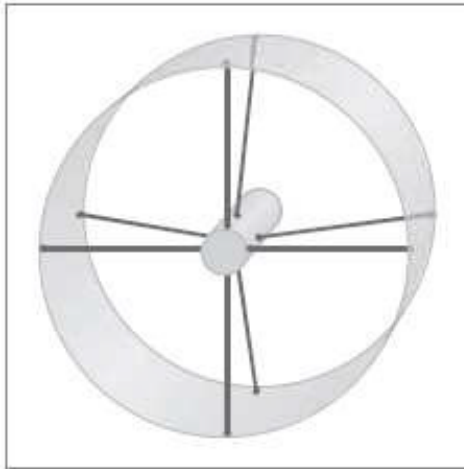
Fig. 12: The wheel is permanently stabilised by internal welded double spokes.
