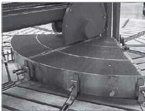
Fig. 11: Large wheels are cut into several segments.
