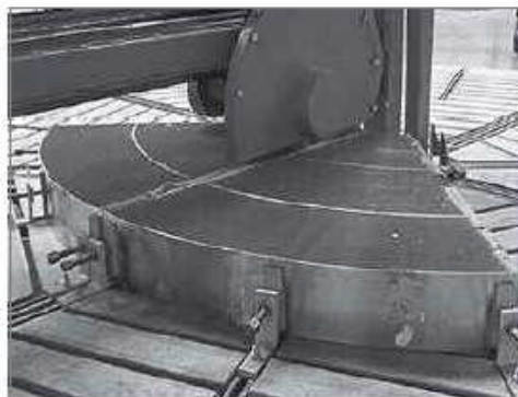
Fig. 11: Large wheels are cut into several segments.
