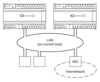
Note: In this configuration IQ4E cannot join a Trend LAN on Ethernet. However, access by IP is still possible.
