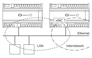
In addition, the IQ4E has the ability to join an internetwork using its virtual INC (see 'Networking' on page 4 for further details).
